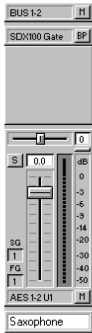
A typical stereo in - mono to stereo out mixer column, as seen within the Mixer.
